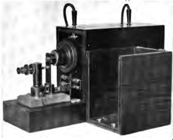
FIG. 21.—Heavy current induction coil for wireless transmitter. [See p. 74.]
